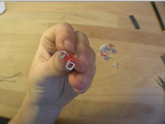
Coil the leads of each LED: make the longer lead (positive) into a square spiral, and the shorter lead (negative) into a round spiral.
